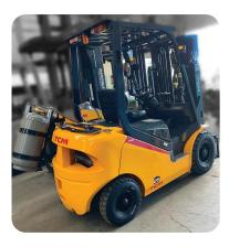
**Easy Gas Tank Change** The LPG cylinder is easily installed and the swing down bracket makes the operator remove the tank in a lower position with minimal effort.
