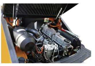
**Wide Opening Engine Hood** Easily accessible engine compartment assures fast and efficient maintenance.
