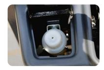
Easy Maintenance Oil Check The T/M oil level can be checked easily without any disassembly.
