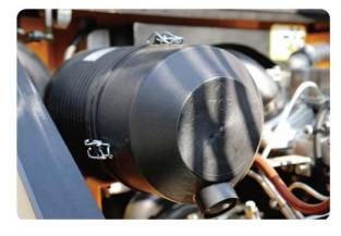
Easy Change of Air Cleaner The air filter is readily accessible for cleaning or replacement. Quick and Easy Engine Oil Check
