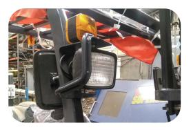
**Excellent Visibility for Safe Operation** Optimized lift cylinder arrangement provides operator with wider visibility, the panoramic mirror expands the driver's view when backing up.
