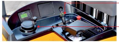
Joystick Controller Finger-operated joystick controller, designed for smooth and precise control
