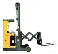
Option of Double Scissors fork: with interlock system for the mast reach and fork reach. (Limited to 9.5M).
