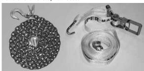
Use a chain with a minimum 3/8 inch diameter and a minimum 7,000 lbs. vertical lift capacity.  Use a strap with a minimum break strength of 10,000 lbs. and a minimum load limit of 3,333 lbs.
